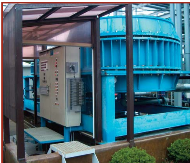
Decationization and Purification Unit (DPU) installed on Capacitor Foil Process in Japan
