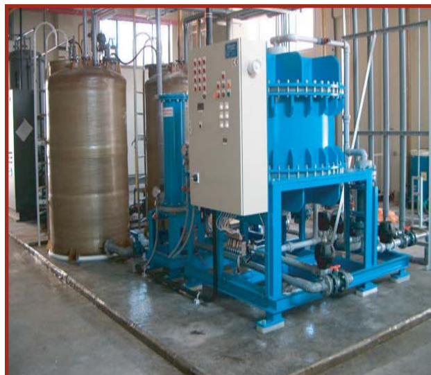
Acid Purification Unit installed on Capacitor Foil Process in Korea
